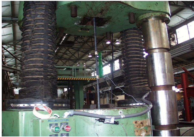
Figure 4-14: Rebar tension test
