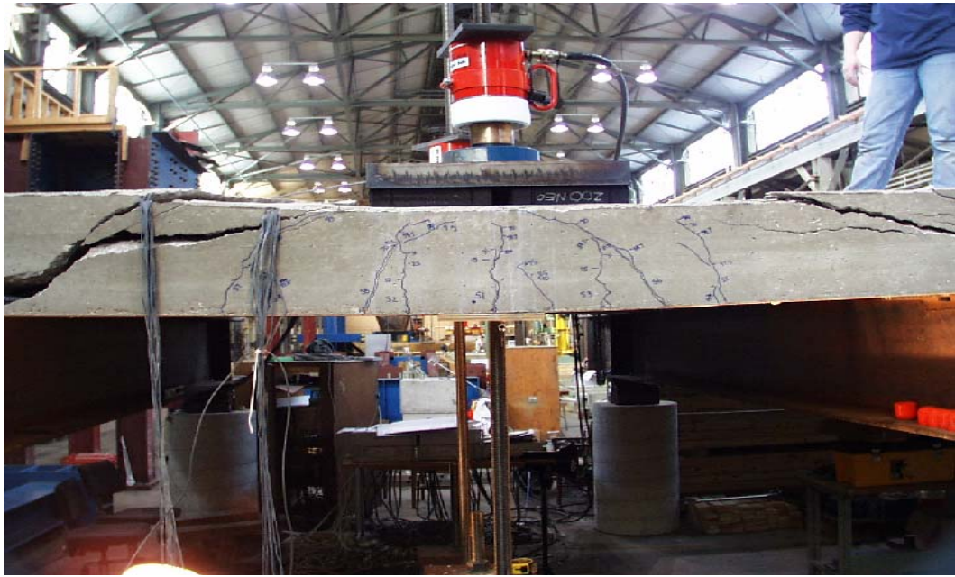
Figure 5-44: Southwest test area failure picture at side of deck, facing north
