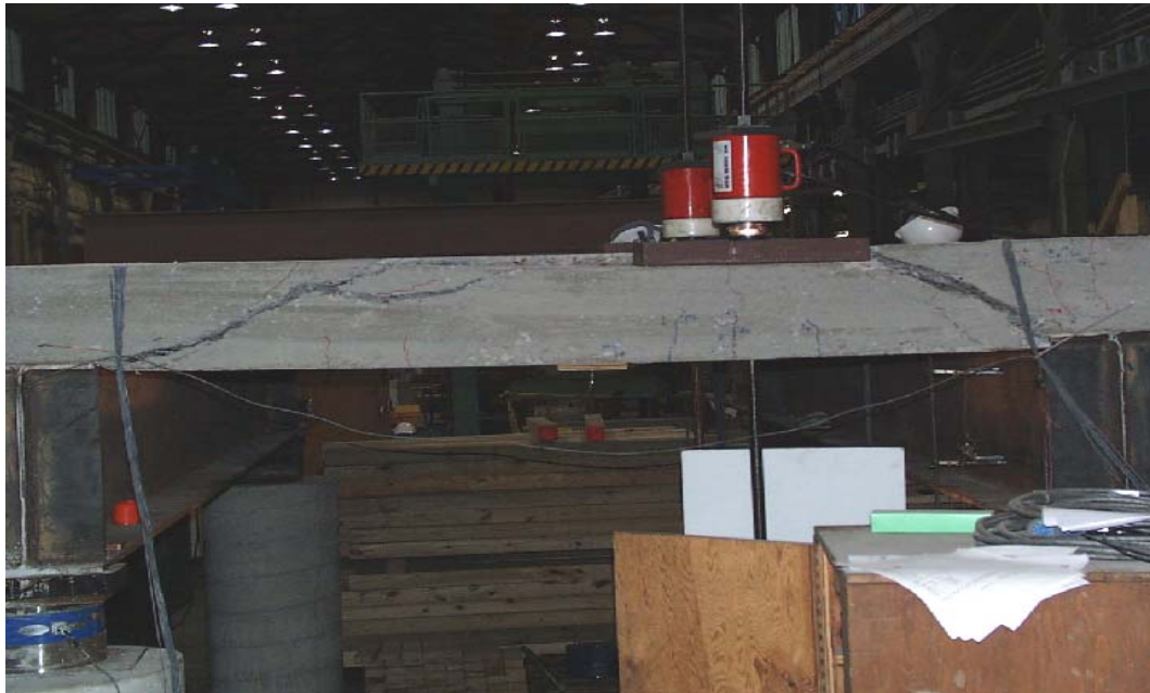
Figure 5-16: Interior span failure at side of deck, interior span, facing north
