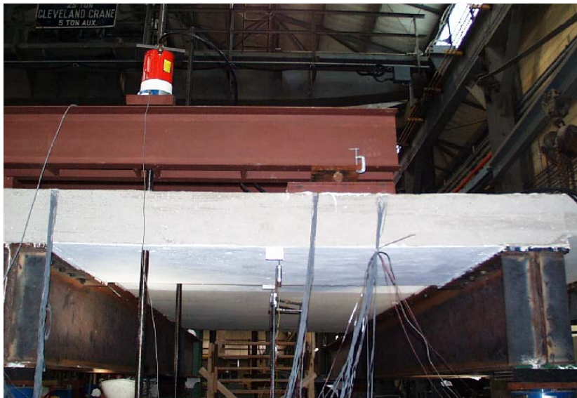
Figure 5-2: Axle loading used to maximize positive moment
