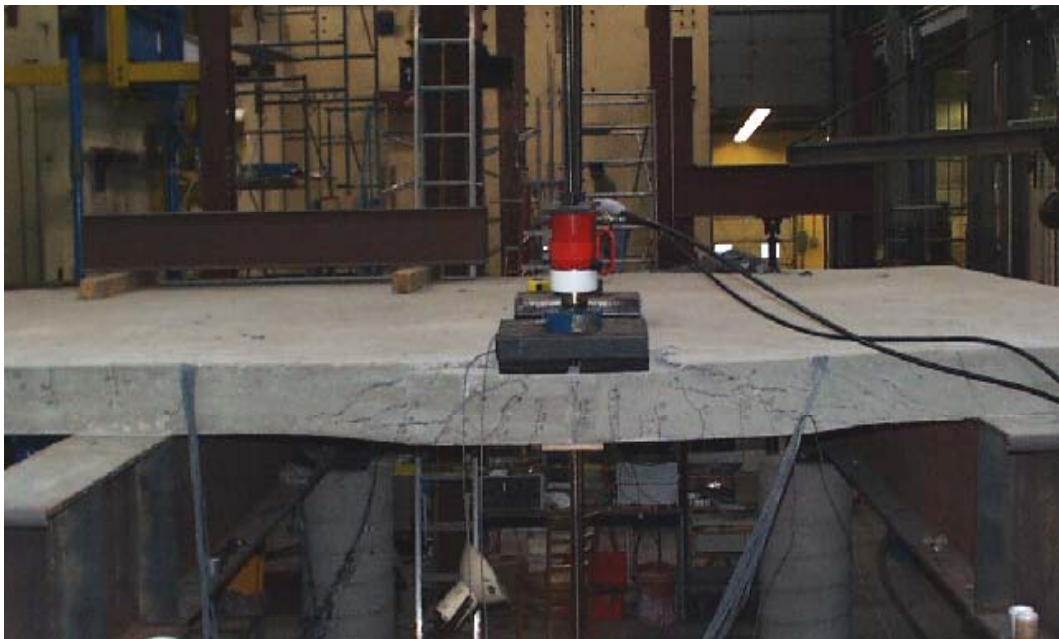
Figure 5-55: Northwest test area failure picture at side of deck, facing south
