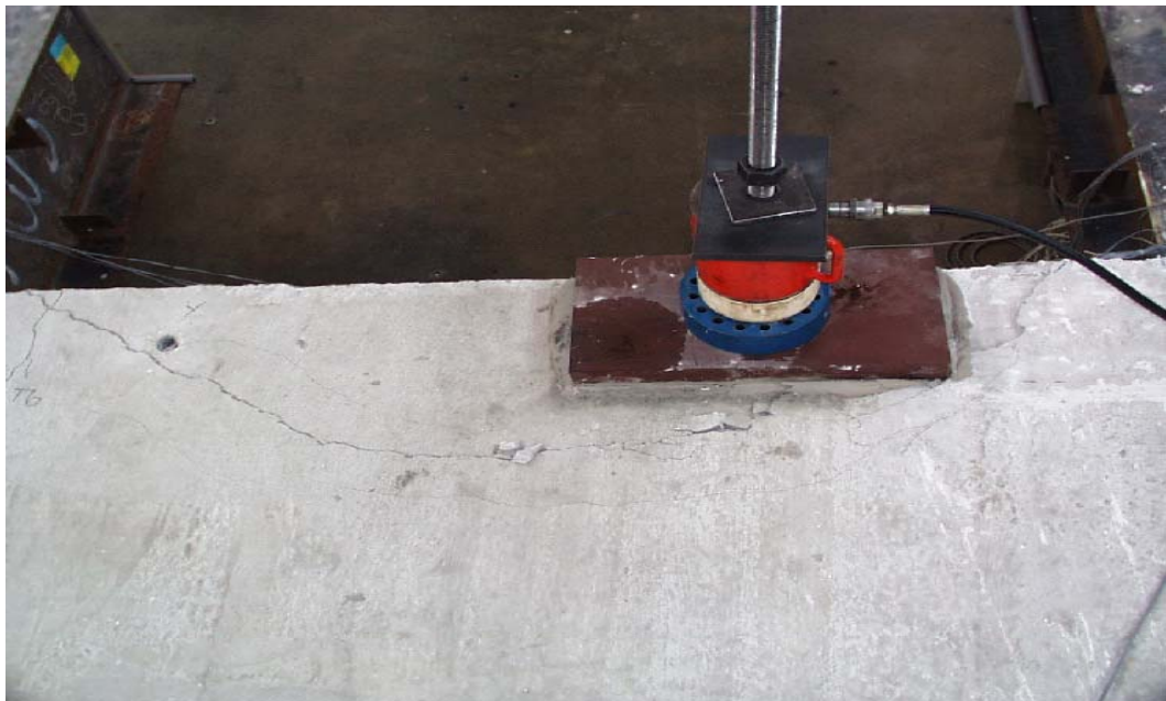
Figure 5-82: Interior span failure at top of deck, facing north
