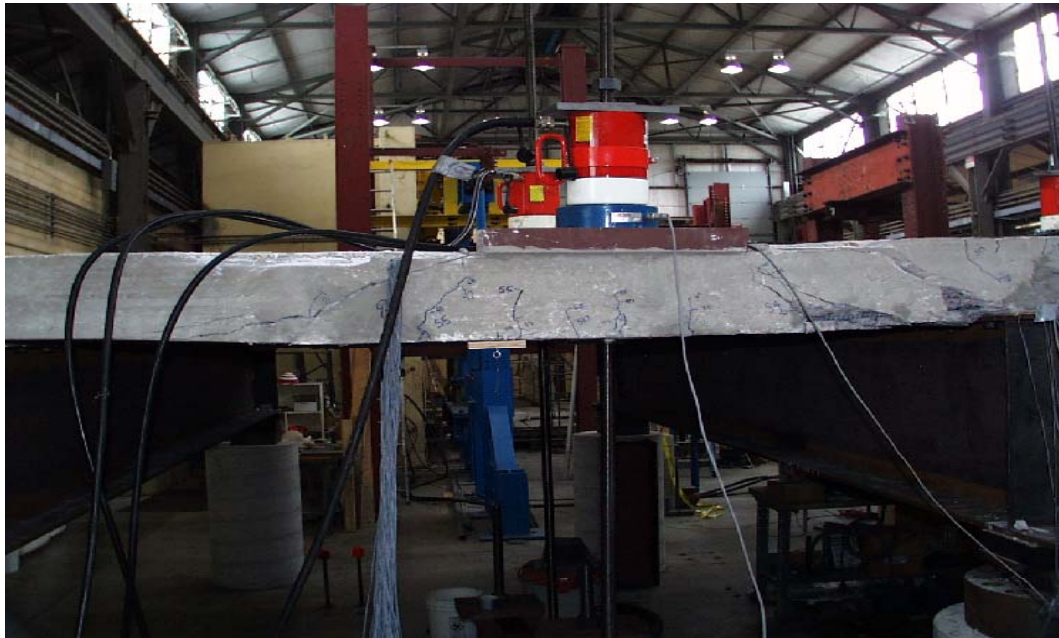
Figure 5-66: Exterior span failure at the side of the deck, interior span, facing south
